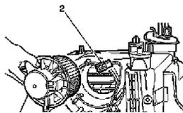
5. Connect the electrical connector (2) to the blower motor (1).
